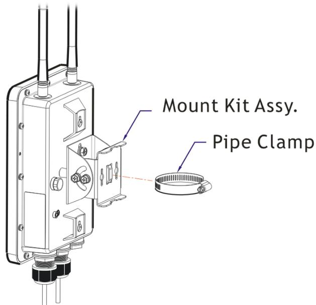
5. Press the pipe clamp to open it for clamping the pole.
