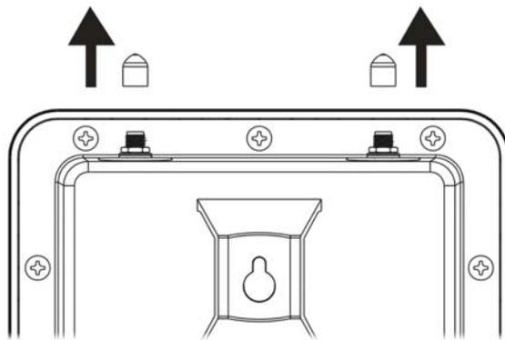
2. Insert the antennas and fasten them by rotating clockwise.
