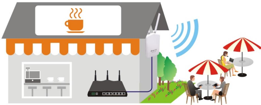
VigorAP 918RPD also is a Power over Ethernet Powered Device which adopts the technology of PoE for offering power supply and transmitting data through the Ethernet cable.
