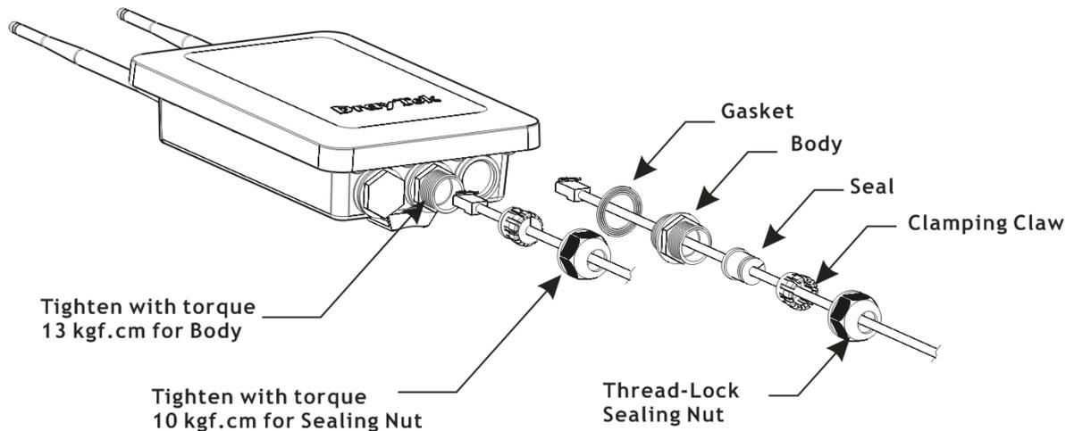
4. Use an adjustable wrench and tighten the thread-lock sealing nut with torque 10 kgf-cm.
