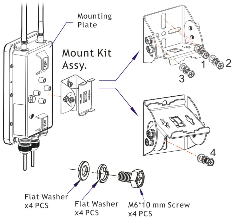
4. Insert the pipe clamp into the mount kit assembly.
